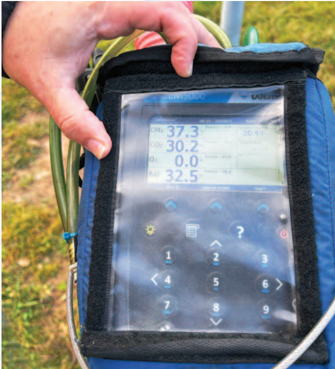
The hand-held GEM5000™ samples and analyzes the methane, carbon dioxide and oxygen content of landfill gas and the results guide adjustments to the suction rates of the gas vacuums attached to each of the active wellheads at the Otter Lake Landfill. Photo: Jason Timms
