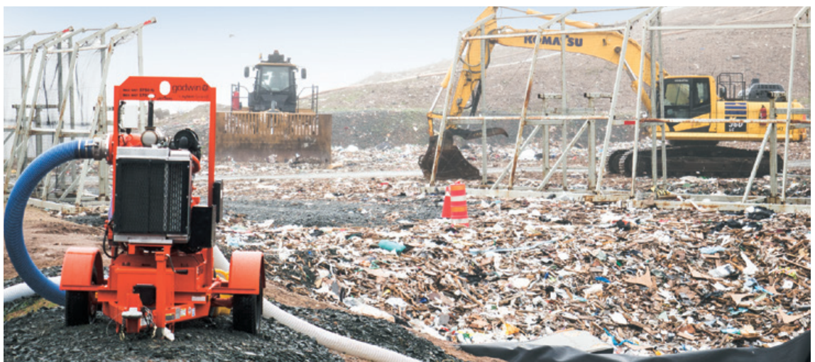
A recent Saturday at Cell 7B, Otter Lake Landfill’s working face, shows idle machinery awaiting the start of the workweek. The white metal screens, vaguely resembling hockey nets, are portable litter fences that move in conjunction with bulldozer operations to protect against flying debris. On windy days, the litter fences are vital.
